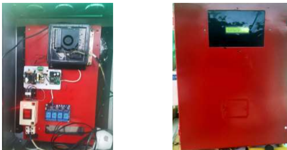
Figure 8. Prototype automation box- inside view ( left ) & outside view ( Right )
