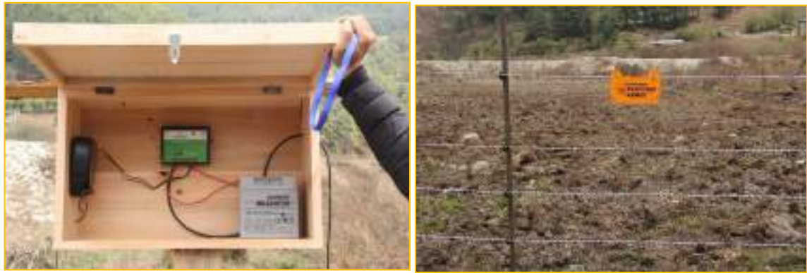
Figure 13. Portable electric fence installed at the pilot site in Bumthang
