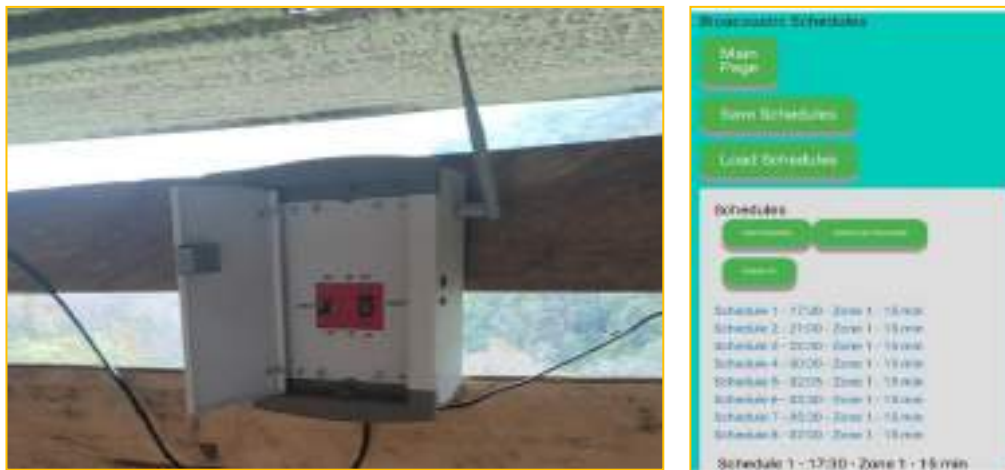
Figure 14. Bioacoustics device (Left) and scheduled time for the bioacoustics system (Right)
