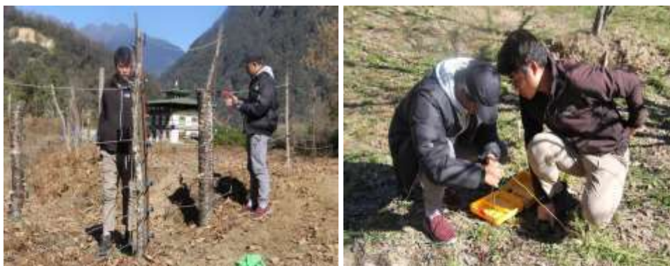
Figure 32. Data collection on the earth resistance (L) and fence voltage of different earthing types (R)
