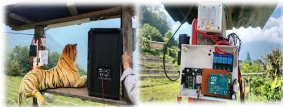
Figure 24. Automated animal repellent installed in field
