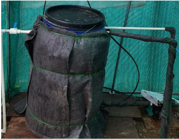
Figure 9. 200 L plastic barrel insulated with black foam to retain water temperature
