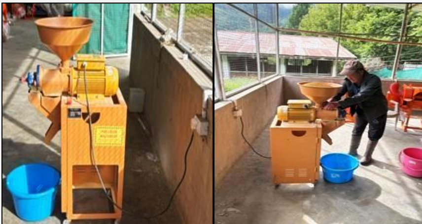
Figure 16: ZLN-4 Rice Mill modified for milling Quinoa to remove saponin.
