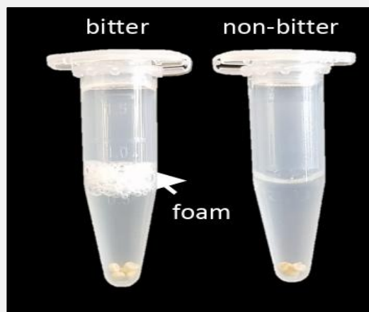
Figure 17: Foam test/ afrosimetric method to quantify saponin in quinoa grain
